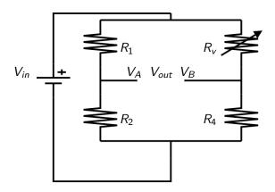
The variable resistor could be in any of the four positions; this is one example.
