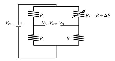
If resistors are chosen to be equal, except for  $R_{\nu}$ , then the output voltage will vary with changes in  $R_{\nu}$ .
