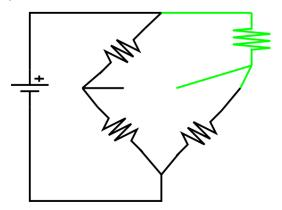
No current flows in measurement lead; similar resistance in both other leads
