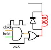
A relay is a device for switching, which is based on a solenoid.
