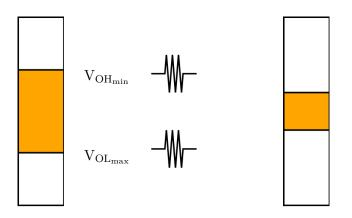
If a signal gets *noise* added to it, the voltage will fluctuate up and down.
