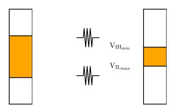
The difference between the output and input limits is the **noise immunity**.
