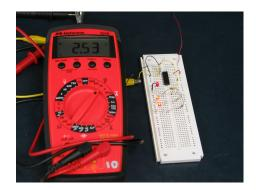
With three LEDs with  $100\Omega$  resistors, the output voltage has dropped further.
