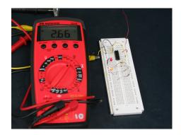
With two LEDs with  $100\Omega$  resistors, the output voltage has dropped further.
