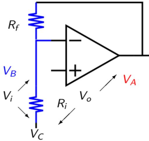
$$V_0 \text{ is } V_A - V_C$$
