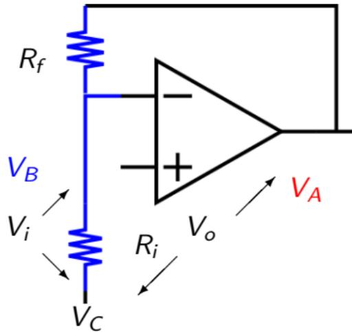
$$V_0 \text{ is } V_A - V_C$$
