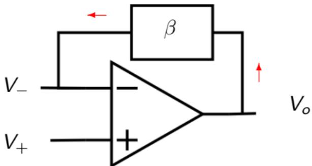
For instance, with just a wire from  $V_-$  to  $V_o$ , the feedabck factor is 1.
