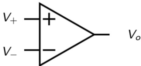
$$V_o = A(V_+ - V_-)$$
