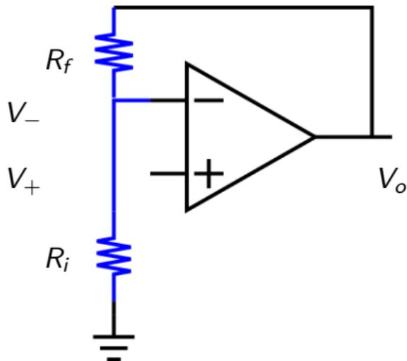
$R_f$  and  $R_i$  form a voltage divider, so the voltage at  $V_-$  is a fraction of  $V_o$
