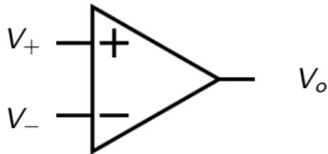
The equation for the output of an op amp is always true *as long as the output is not saturated*
