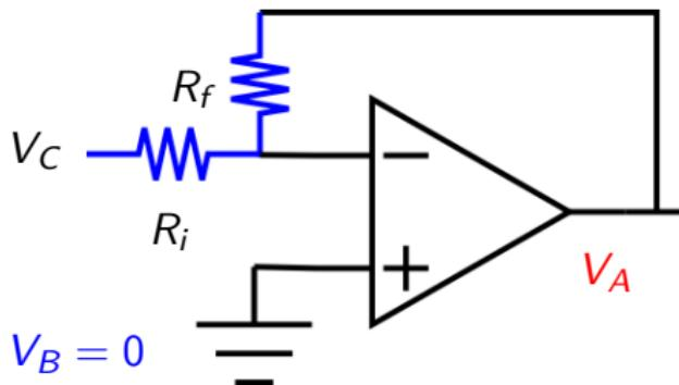
$$\text{So if } V_A - \left(1 + \frac{R_f}{R_i}\right) V_B = -\frac{R_f}{R_i} V_C$$
