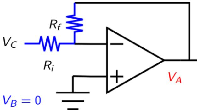
$$\text{So if } V_A - \left(1 + \frac{R_f}{R_i}\right) V_B = -\frac{R_f}{R_i} V_C$$
