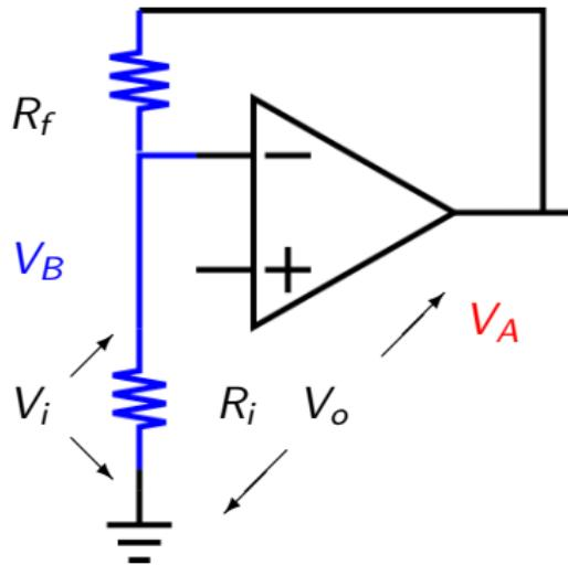
$$\frac{V_o}{V_i} = \frac{V_A}{V_B} = 1 + \frac{R_f}{R_i}$$
