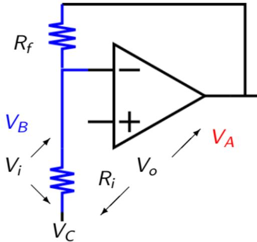
$$V_0 \text{ is } V_A - V_C$$
