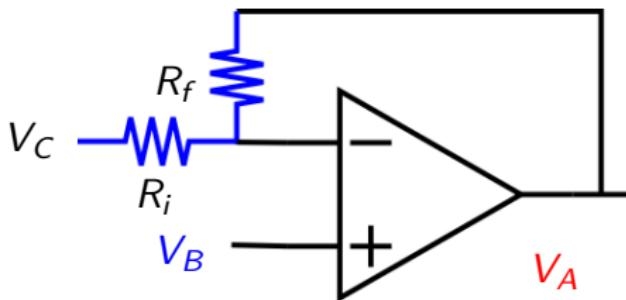
$$\text{Since } \frac{V_A - V_C}{V_B - V_C} = 1 + \frac{R_f}{R_i}$$
