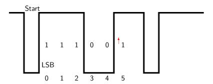
Wait one bit time before testing pin for bit 5
