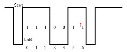
Wait one bit time before testing pin for bit 6
