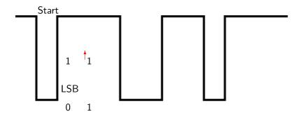
Wait one bit time before testing pin for bit 1
