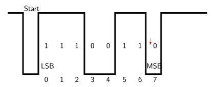
Wait one bit time before testing pin for MSB
