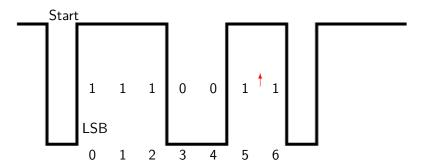
Wait one bit time before setting pin HIGH or LOW according to bit 6
