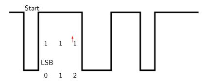
Wait one bit time before testing pin for bit 2
