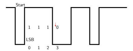
Wait one bit time before testing pin for bit 3
