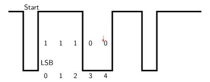
Wait one bit time before testing pin for bit 4
