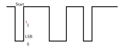
Wait one and a half bit times before testing pin for LSB
