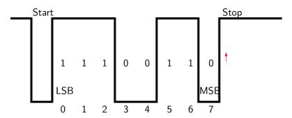
Wait one bit time before testing pin for STOP level
