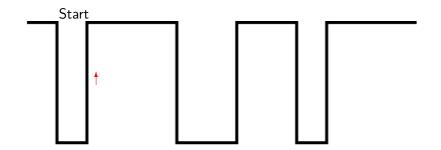
Wait one and a half bit times before testing pin for LSB
