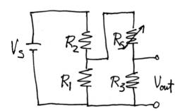
4. Assuming the resistive sensor in the above circuits is a photoresistor, explain the difference in operation of the above circuits.
