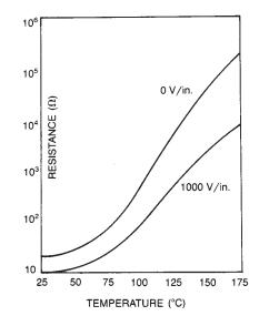
Figure 24: Voltage Dependence of PTC's.
