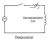
Figure 28: Time Delay, Motor Start, Degaussing.
