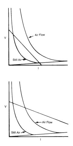
Figure 30: Flow Sensor / Liquid Level.
