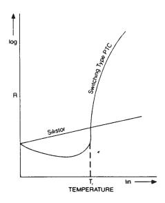
Figure 22: R-T Characteristics of PTC Thermistors.
