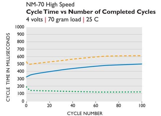
Increasing the applied voltage heats the device more quickly enabling the device to cycle faster.
