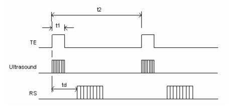
Figure II.1 Basic Operation Timing
