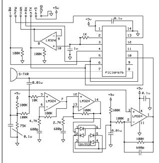
250mS after power-up, the LV-MaxSonar<sup>®</sup>-EZ0<sup>TM</sup> is ready to accept the RX command. If the RX pin is left open or held high, the sensor will first run a calibration cycle (49mS), and then it will take a range reading (49mS). Therefore, the first reading will take ~100mS. Subsequent readings will take 49mS. The LV-MaxSonar<sup>®</sup>-EZ0<sup>TM</sup> checks the RX pin at the end of every cycle. Range data can be acquired once every 49mS.
