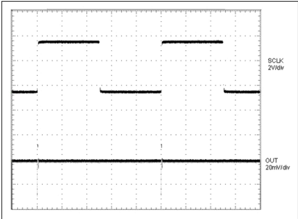
Figure 3. Digital Feedthrough
