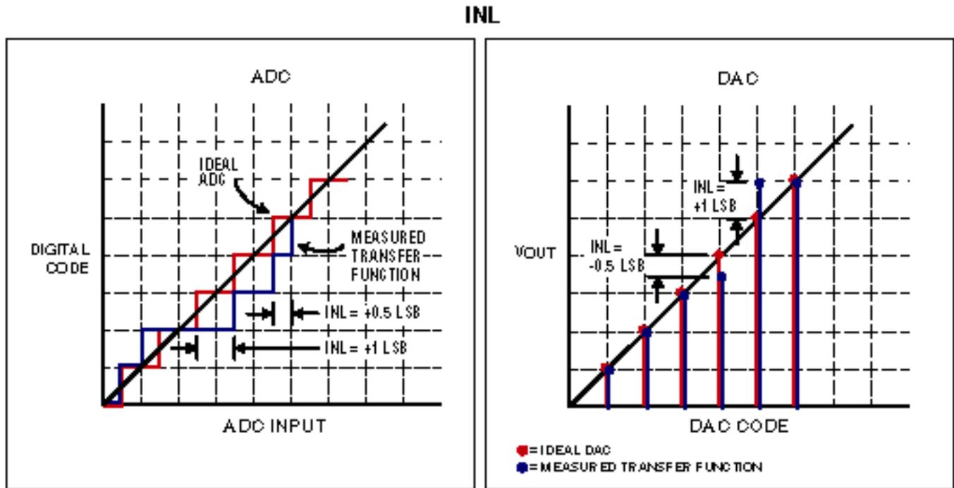
Figure 6. INL for a) ADC and b) DAC
