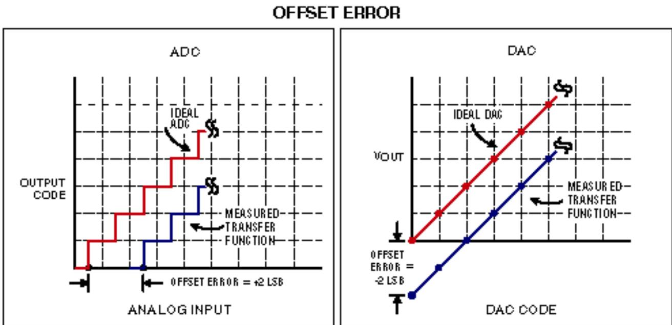
Figure 7. Offset Error for a) ADC and b) DAC
