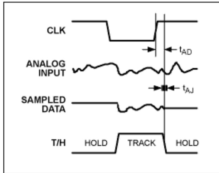
Figure 1. Aperture Delay and Jitter
