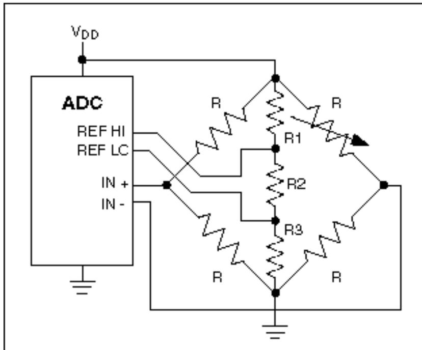
Figure 8. Ratiometric Measurement Using Resistive Bridge Network resolution
