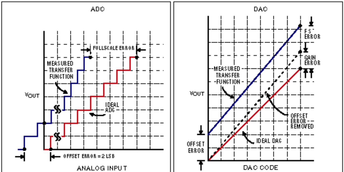
Figure 4. Full-Scale Error for a) ADC and b) DAC
