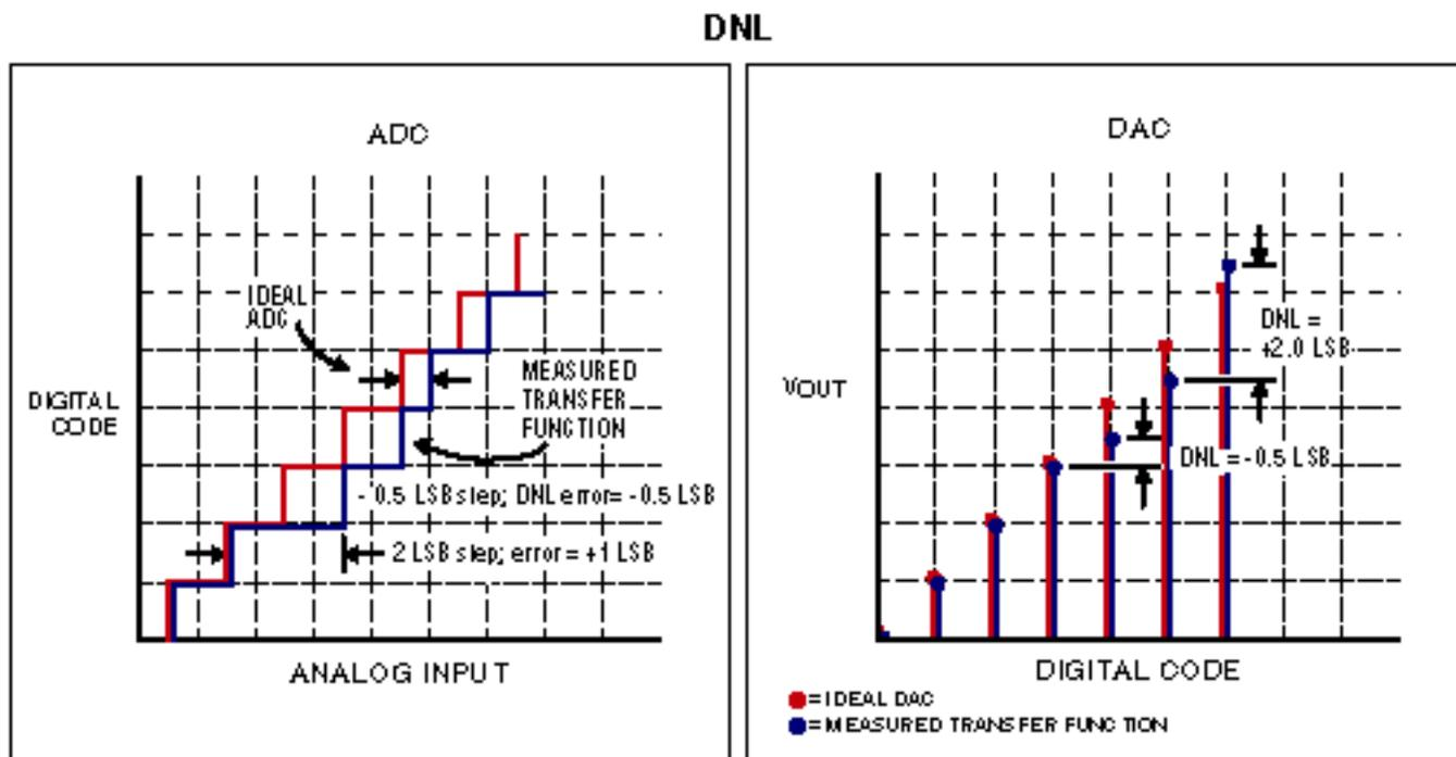
Figure 2. DNL for a) ADC and b) DAC
