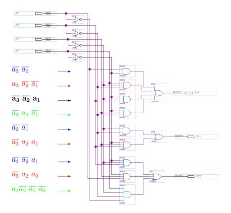
The terms for each of the outputs are identified, and the corresponding gates are colour-coded in the same way to make it easy to identify each gate with its corresponding AND term in an equation.
