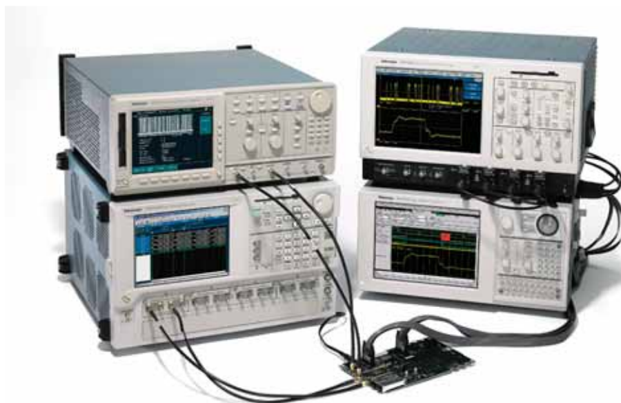
► Figure 1. Most measurements require a solution made up of a signal source paired with an acquisition instrument. Triggering connectivity simplifies capturing of the DUT output signal.
