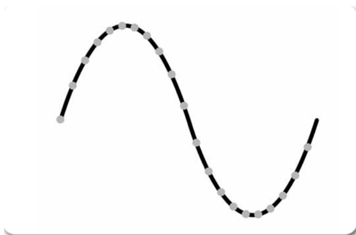
► Figure 17. (Left) A series of sampled points representing a sine wave; (Right) the reconstructed sine wave.
