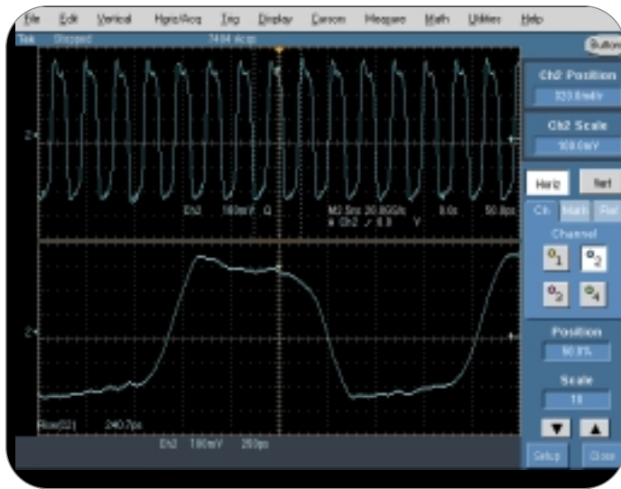
► Figure 48. Rise time characterization of a high-speed digital signal.
