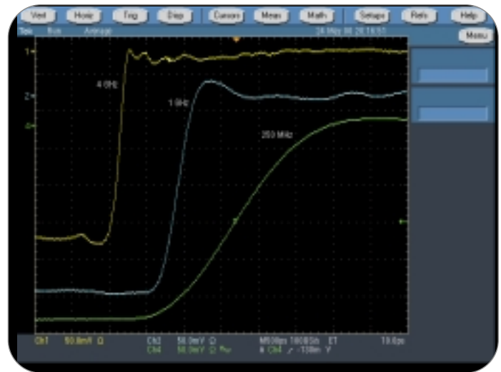
▶ Figure 47. The higher the bandwidth, the more accurate the reproduction of your signal, as illustrated with a signal captured at 250 MHz, 1 GHz and 4 GHz bandwidth levels.
