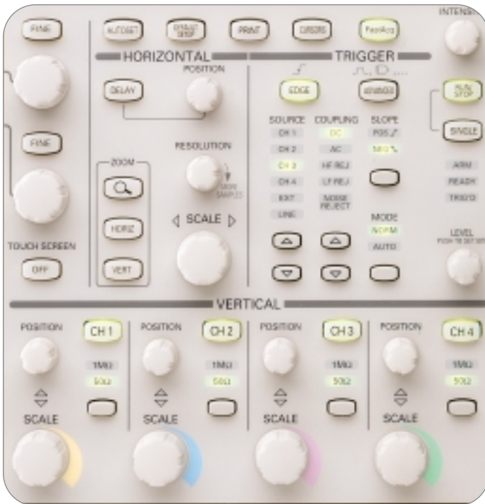
► Figure 22. Front-panel control section of an oscilloscope.
