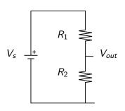
$$V_{out} = V_s \left( rac{R_2}{R_1 + R_2}
