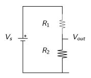
If  $R_1$  gets *smaller*, then  $V_{out} = V_s \left( \frac{R_2}{R_1 + R_2} \right)$  gets *bigger*.
