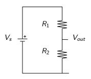
Since  $I_1=I_2$ , (by Kirchhoff's current law), and  $V_s=V_{R_1}+V_{R_2}$ ,
