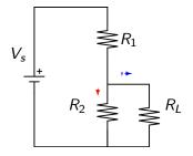
Some current goes through  $R_2$ , but some goes through  $R_L$  so the *effective* value of  $R_2$  is reduced.
