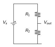
Since  $I_1=I_2$ , (by Kirchhoff's current law), and  $V_s=V_{R_1}+V_{R_2}$ , (by Kirchhoff's voltage law), so  $V_s=I_1R_1+I_1R_2=I\left(R_1+R_2\right)$   $I=\frac{V_s}{R_1+R_2}$
