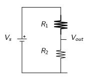
If  $R_1$  gets bigger, then  $V_{out} = V_s \left( \frac{R_2}{R_1 + R_2} \right)$  gets smaller.
