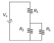
Load will reduce the output voltage
