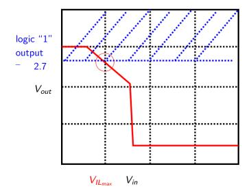
Real logic gates Measuring voltage limits
