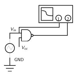
Real logic gates Measuring voltage limits
