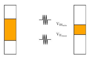
The difference between the output and input limits is the **noise immunity**.
