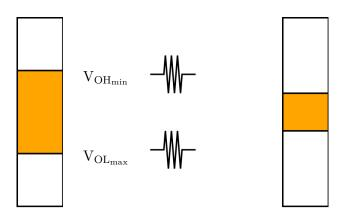
If a signal gets *noise* added to it, the voltage will fluctuate up and down.
