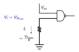
The current *limit* is when  $V_i = V_{IL_{max}}$ .
