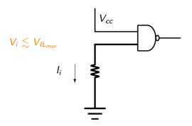
Some resistance will allow enough current to make the input  $V_{IL_{max}}$ .
