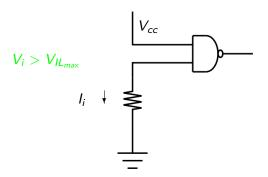
A large resistor won't allow enough current to make the input LOW.
