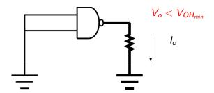
A low enough resistance will allow enough current to make the output below  $V_{OH_{min}}$ ; i.e. invalid as a HIGH.
