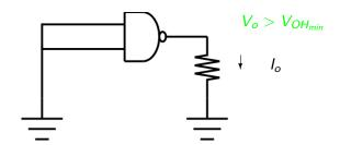
A large resistor won't allow enough current to keep the output from being a valid HIGH.
