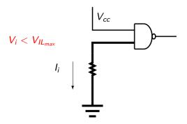
A low enough resistance will allow enough current to make the input below  $V_{IL_{max}}$ ; i.e. LOW.
