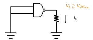
Some resistance will allow enough current to make the output  $V_{OH_{\min}}$ .
