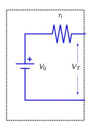
The potential difference between the terminals of a battery,  $V_T$ , decreases as the current supplied by the battery increases.
