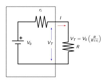
$$V_T = V_0 \left( \frac{R}{R + r_i} \right)$$
