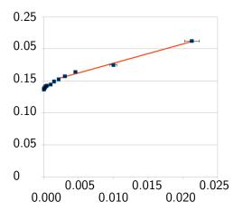
The steeper slope of this graph compared to the last one indicates that the internal resistance is much higher; in other words, the output voltage changes much more as current increases compared to the new battery.
