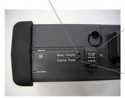
DC input connector Used to connect the supplied AC adapter.
