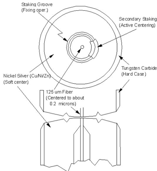
**Figure 1-3. Cross-section of the Diamond HMS-10 connector.**
