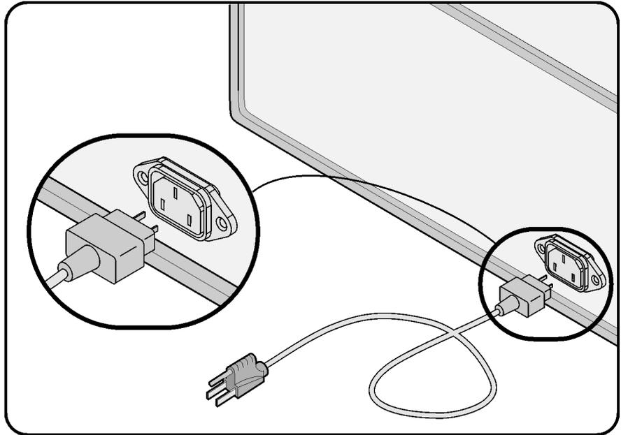
The Infiniium DCA automatically adjusts for line input voltages in the range of 100 to 240 VAC. There is no manual selection switch. The line cord provided is matched by Agilent to the country in which the order originates. Refer to [Table 1-8, "Available Line Cords," on page 1-12](#) for a list of available line power cords.
