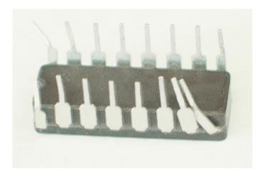
Again, the direction is clear by the way the pins are bent.
