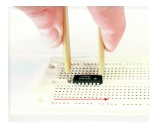
Put the jaws of the chip puller over the ends of the chip.
