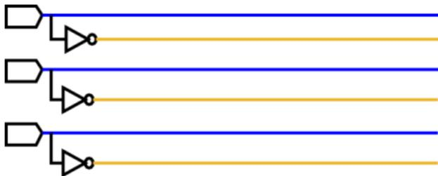
For each input, add an inverter as shown and add wires, as with the inputs.
