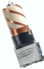
Figure 4 – Sarantel helix antenna (cover removed)
