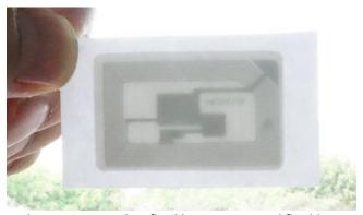
It also supports reading flexible tag. We tested flexible tags of Mifare 1 S50 and Ultralight. The reading distance is up to 5cm.
