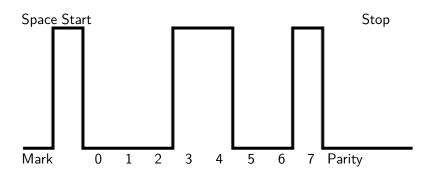
Serial Communication -UART Arduino Serial Library Baud rate calculation RS232 communication
