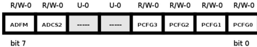
Bits in ADCON1 register - Note ADCS2
