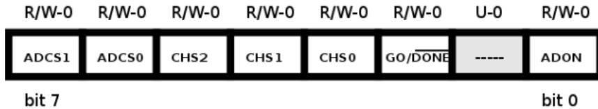
Bits in ADCON0 register - Note ADCS1, ADCS0
