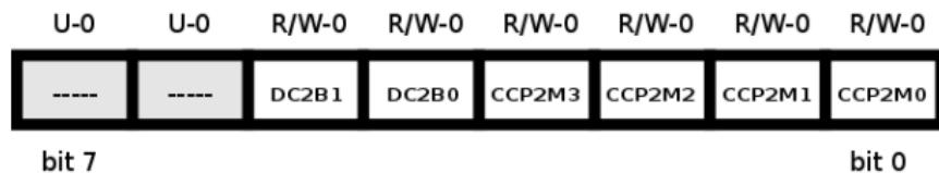
Bits in CCP2CON register -Mode 1011 can start ADC
