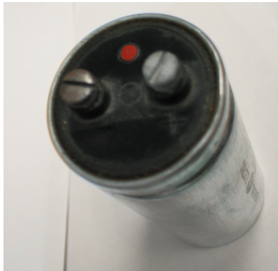
Big electrolytic capacitor (top view)
